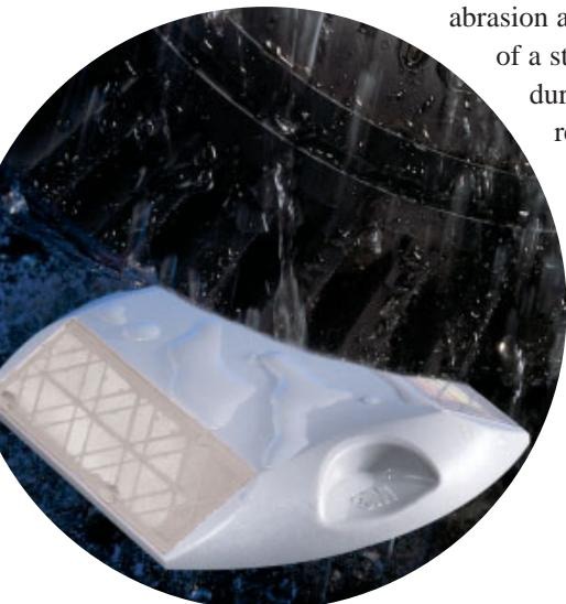
*The Series 290 stud gives maximum impact resistance. When tested according to ASTM standards, the marker body displays no cracking or breakage using a 1000 gm weight from a height of 1 metre.*
