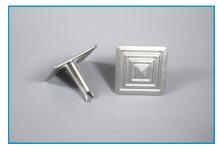
The stainless steel crossing studs are also 100mm square and have a serrated finish to improve skid resistance in adverse weather conditions, and have a fishtail shank.
